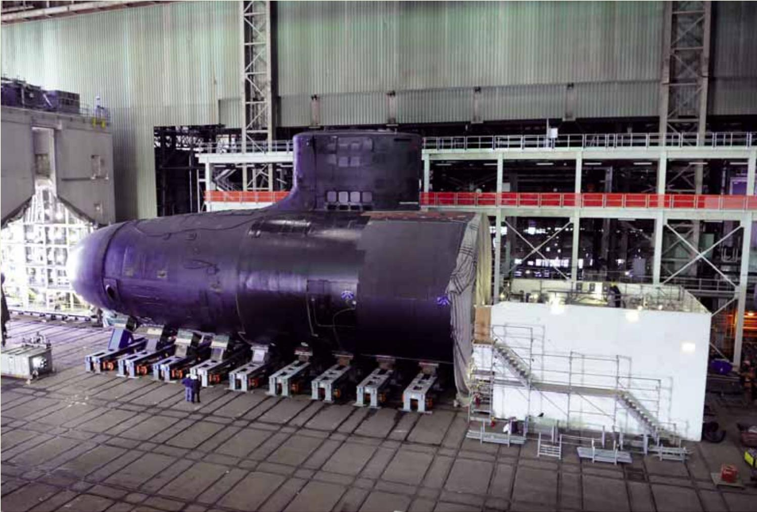
A view of the forward end of the submarine Missouri (SSN-780) from one of the work platforms built to improve construction efficiency in Building 260.
